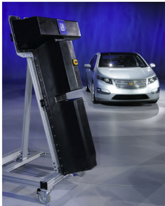
Fig. 6. GM Volt car and battery. The battery that powers the Chevy Volt occupies a significant fraction of the volume of the car. A full charge enables driving 38 miles.
